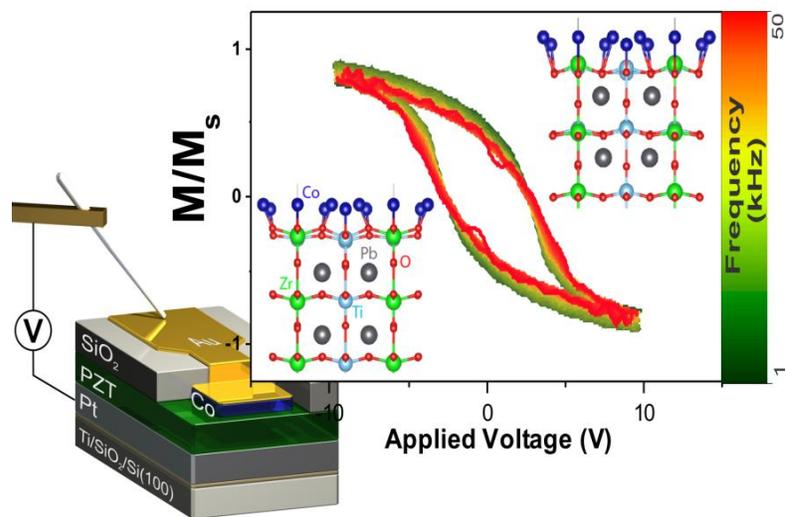
**Figure |** A rectangular magnetoelectric hysteresis loop is obtained in Co/PbZrTiO<sub>3</sub> bilayers. This hysteretic behavior traduces the existence of two magnetization states corresponding to two opposite voltage values. Moreover, the two states do not vanish when the voltage is switched off. [Vla16]
